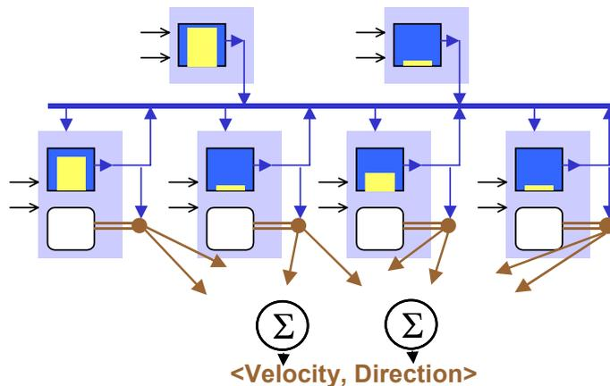
**Figure 2.** The behavior hierarchy in Dual Dynamics.
