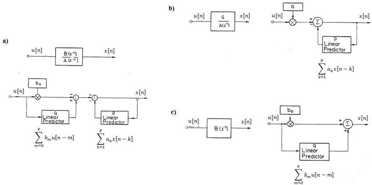
Figure 5-2: Block diagram of a) ARMA model, b) AR model and c) MA model in time domain and their z-transform [1].
