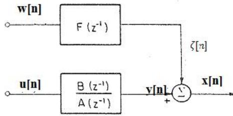
Figure 5-1: The transfer function model [1].
