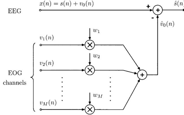
Figure 5-8: Cancellation of eye movement artifact based on linear combination of EOG signals using the fixed weights [2].
