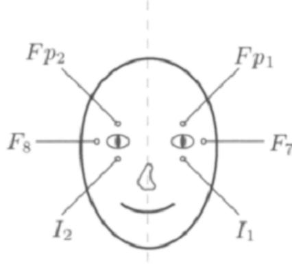
Figure 5-7: Electrode positions for recording EOG signals which reflects horizontal ( $F_7 - F_8$ ) and vertical eye movement ( $Fp_1 - I_1$  or  $Fp_2 - I_2$ ) [2].
