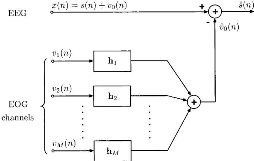
Figure 5-12: Cancellation of eye movement artifacts using an estimate based on linear FIR filtering of  $M$  different EOG channels [2].
