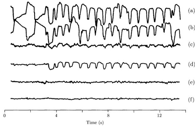
Figure 5-9: An example of EOG artifact cancellation in EEG signals. a,b) EOG signals measured for right and left eyes. c,d) EEG signals from two different electrodes before and e,f) after artifact cancellation [2].
